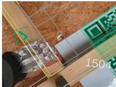
Figure 2: Positioning-outlines, localisation marker, release button and object ID
