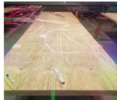
Figure 14: Projection of the outlines via AR device
