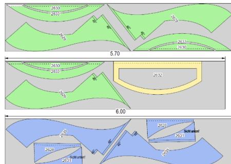
Figure 13: Placement of the curves within the measurements of the sheets
