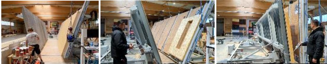
Figure 6: Sequence of butterfly turning table in action
