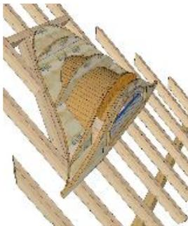
Figure 12: 3D geometry of a bat dormer
